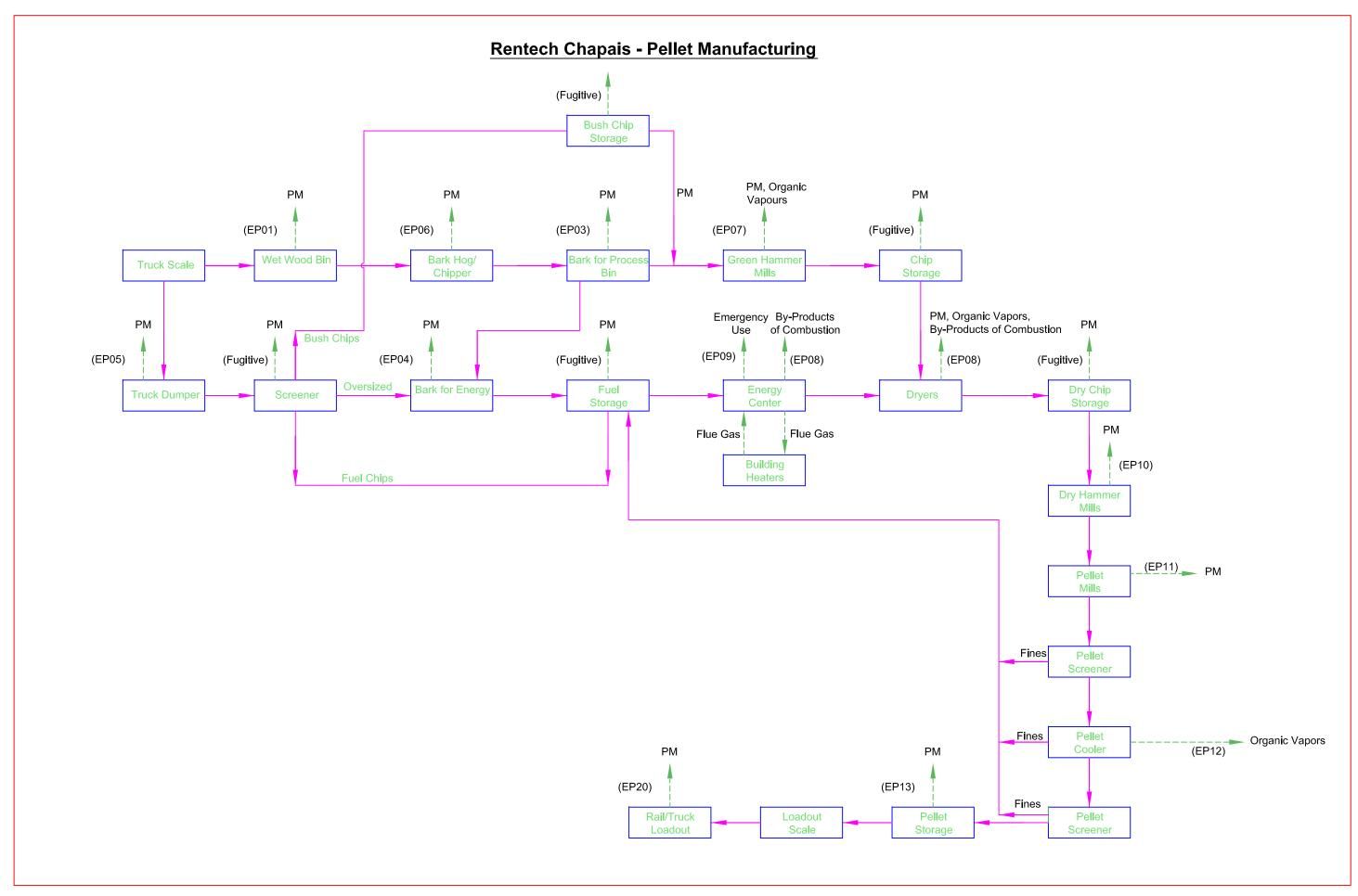
Figure B1a: Process Flow Diagram
