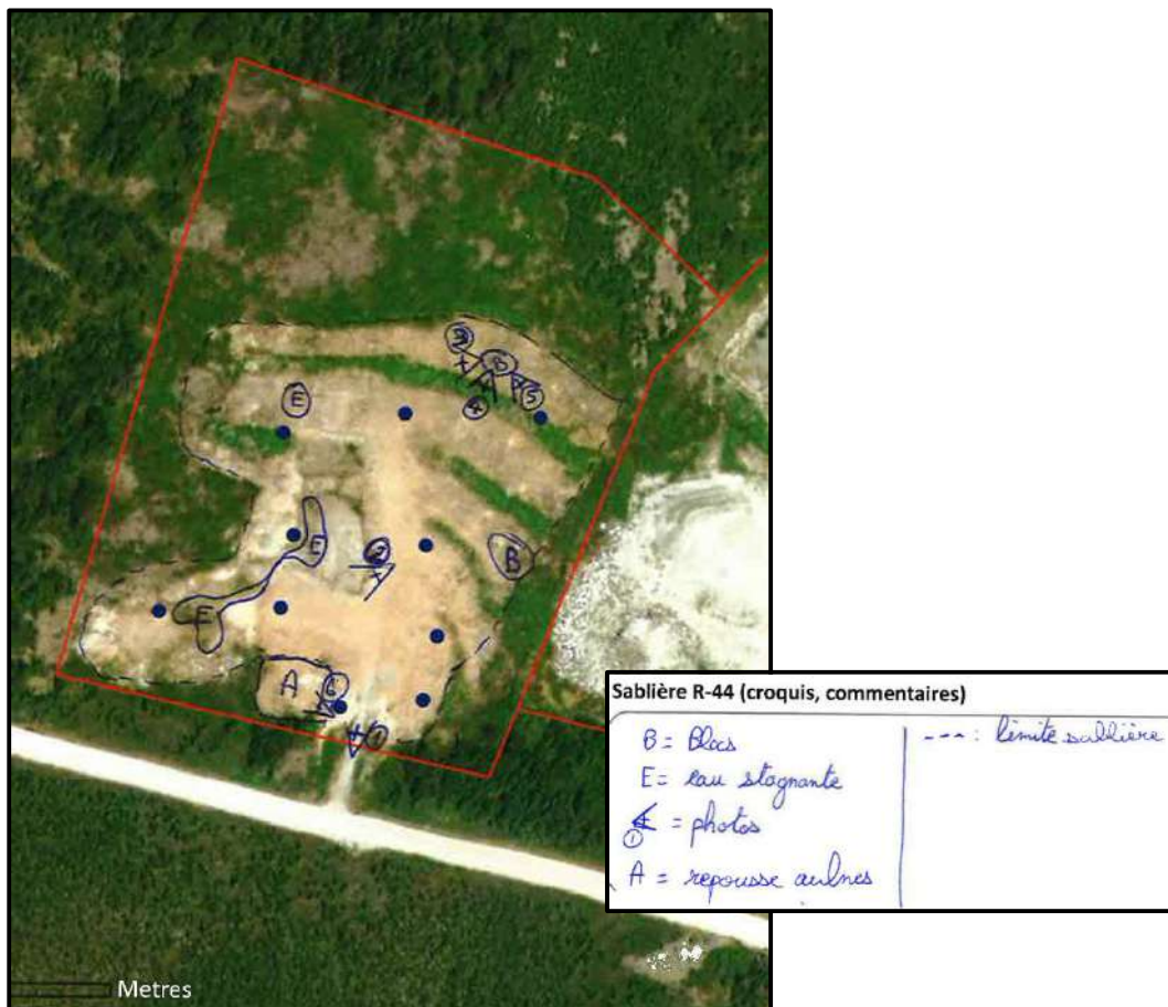
Figure 14: Aerial photo of Sand Pit R-44 and summary of the characteristics observed (Sand Pit Sampling Report, 2020-06-28)
