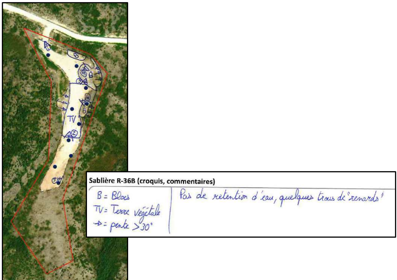
Figure 12: Aerial photo of Sand Pit R36-B and summary of the characteristics observed (Sand Pit Sampling Report, 2020-06-28)
