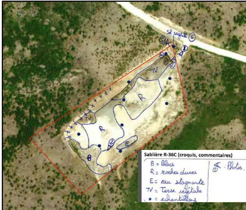
Figure 9: Aerial photo of Sand Pit R36-C and summary of the characteristics observed (Sand Pit Sampling Report, 2020-06-28)
